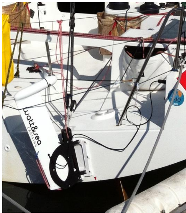
Lifting the hydrogenerator
