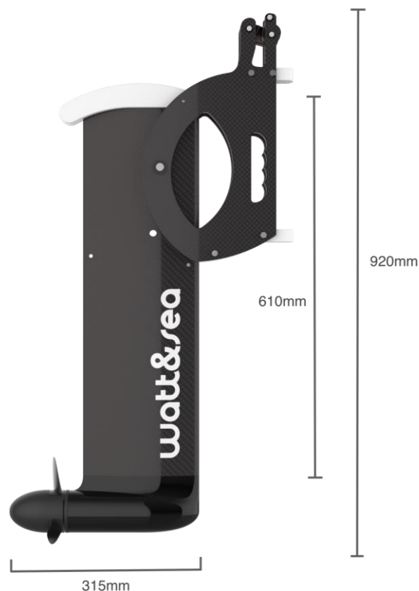
Dimensions of the Class 40 hydrogenerator
